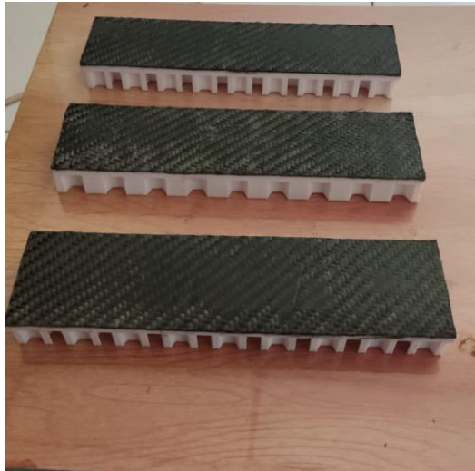
Gambar 3- 34 Hasil Proses Vacuum Bagging
