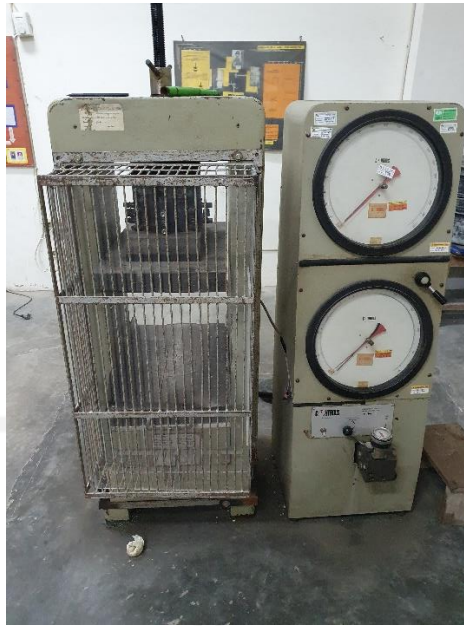
Gambar L-3.13 Compressing Testing Machine (CTM)
