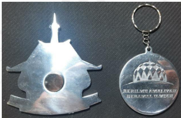
Gambar 4.20 Hasil finishing tampak belakang
