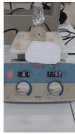
Wet Peroxide Oxidation
