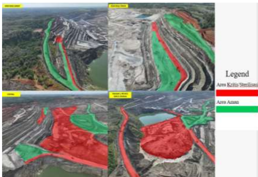
Gambar 3. Geotechnical Map of Concern Area/Geotechnical Hazard Map
