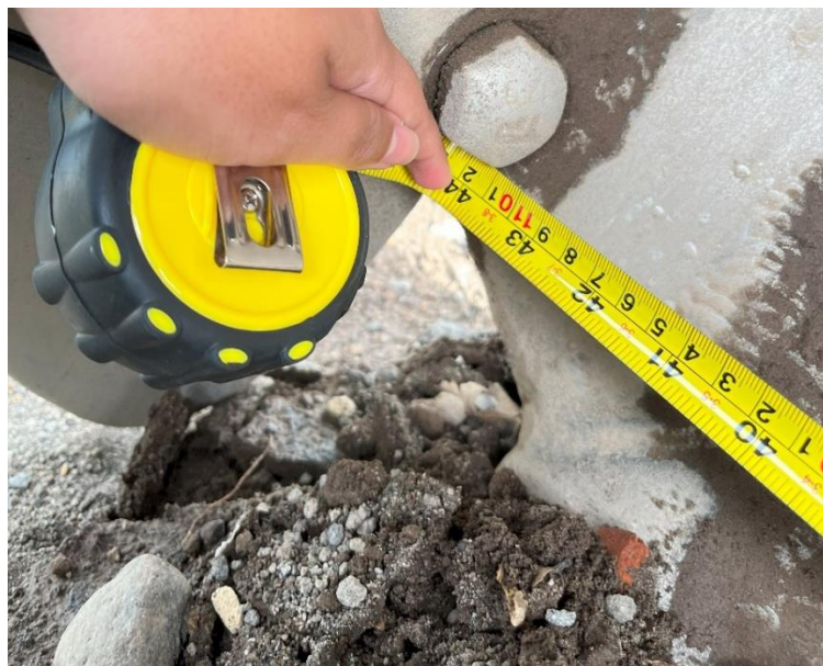
Gambar 5.8 Lebar Bucket Excavator Komatsu PC200 113 cm
