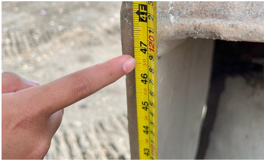
Gambar 5.9 Panjang Bucket Excavator Komatsu PC200 120 cm
