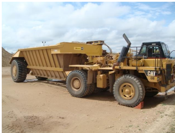
Gambar 3.5 Bottom Dump Truck
