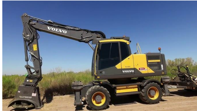
Gambar 3.2 Wheel Mounted Excavator
