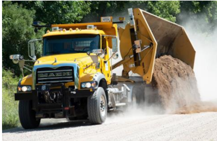
Gambar 3.4 Side Dump Truck
