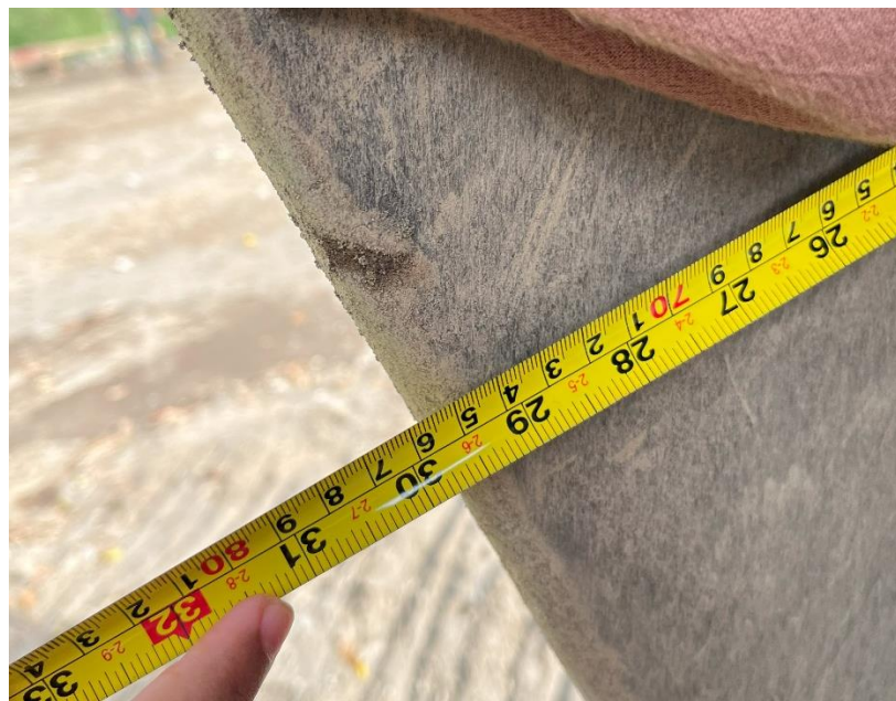
Gambar 5.10 Kedalaman Bucket Excavator Komatsu PC200 75 cm
