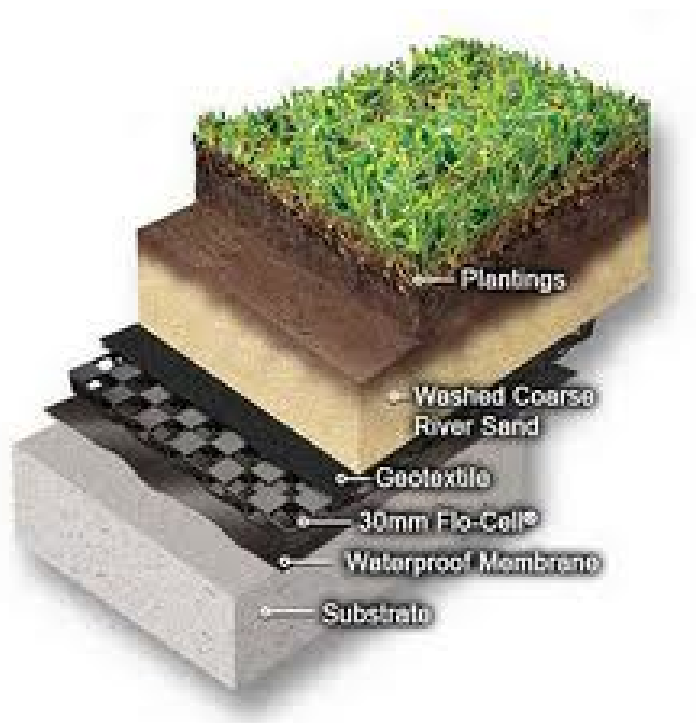
Gambar 3.32. Lapisan Roof Garden
