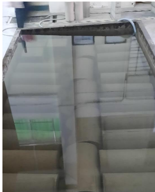
Gambar 3. 8 Proses Perendaman Beton
