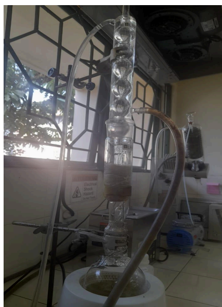
Gambar 3.5 Sokletasi Substrat Jerami
