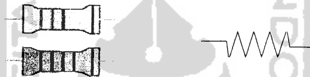
Gambar 2.3 a)Resistor b)Simbol Resistor
