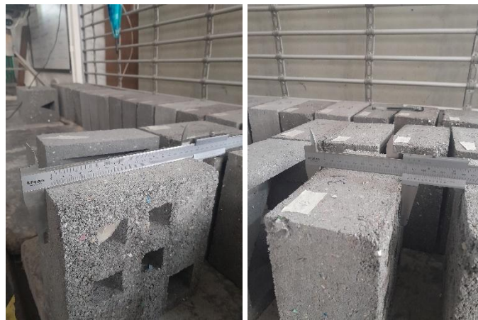
Gambar 4. 3 Pengukuran Roster Beton
