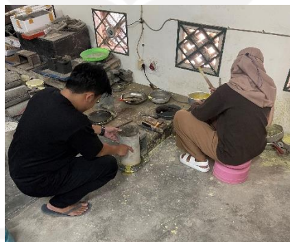
Gambar L.11.7 Proses Capping Benda Uji
