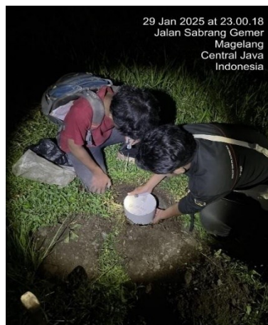
Gambar 5.2 Proses Leveling Seismometer
