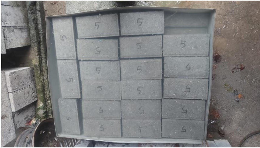
Gambar L-5.4 Proses Perawatan Paving Block
