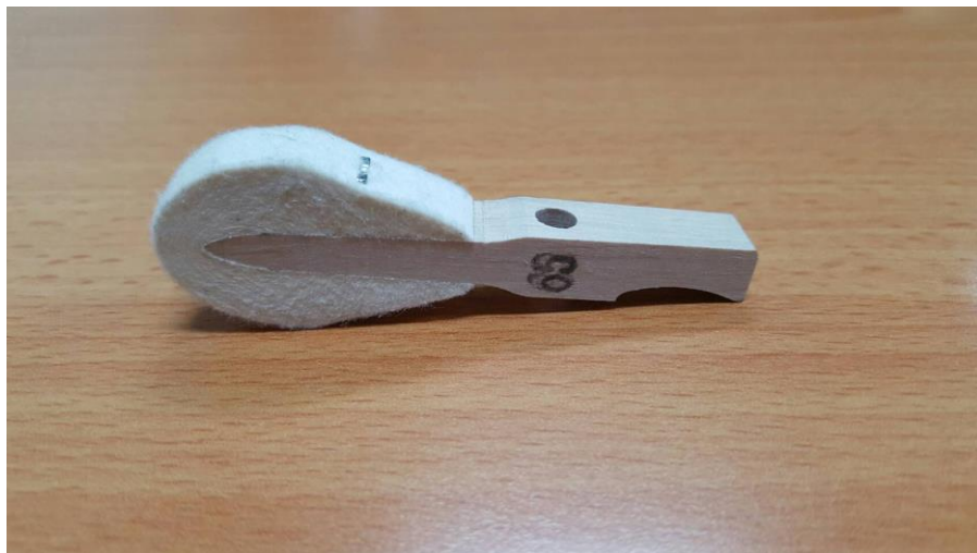
Gambar 1.2 Kabinet Hammer Head
