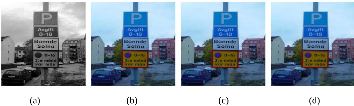
Gambar 2.6 (a) Histogram equalization , (b) Compression , (c) Normalization , (d) Noise reduction ,
