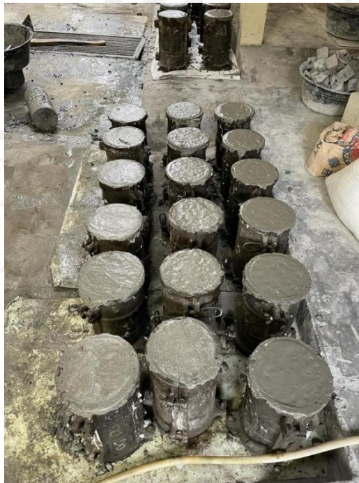
Gambar L-1.12 Beton Segar Pasca Mixing
