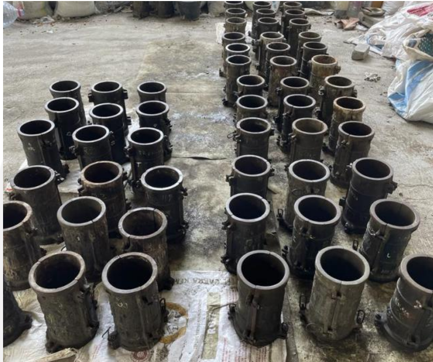
Gambar L-1.9 Persiapan Bekisting Sebelum Mixing
