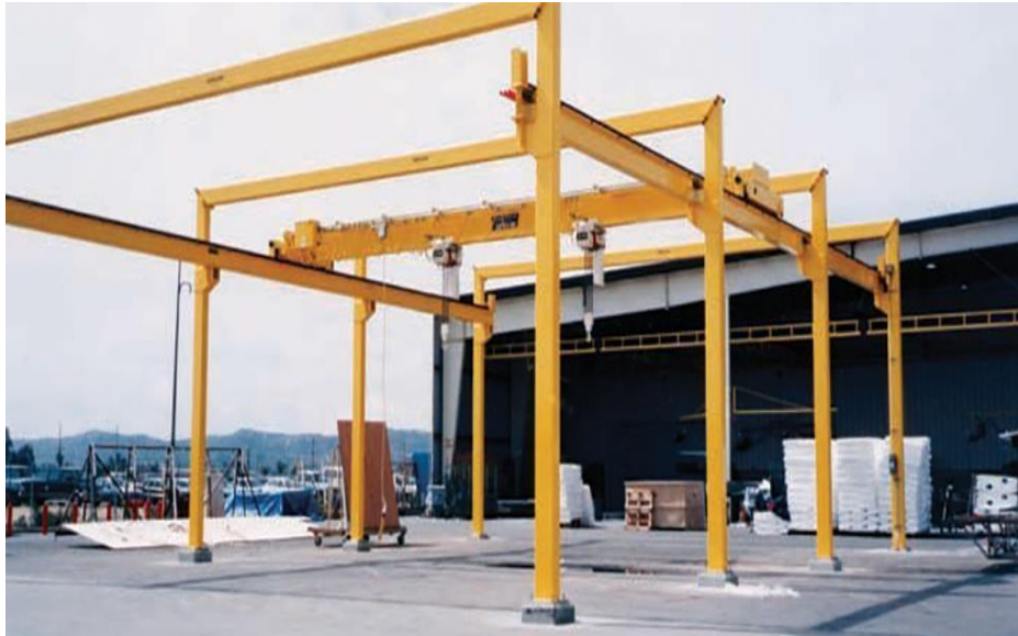
Gambar 3.1 Free Standing Crane (Sumber : Proservcrane.com )
