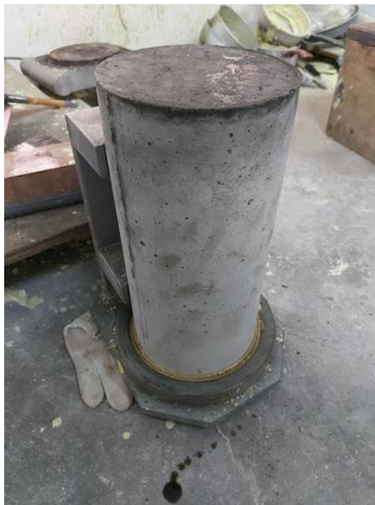
Gambar L-10.12 Proses Capping Beton
