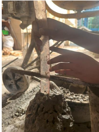
Gambar 5. 10 Uji Slump Trial Mix Design
