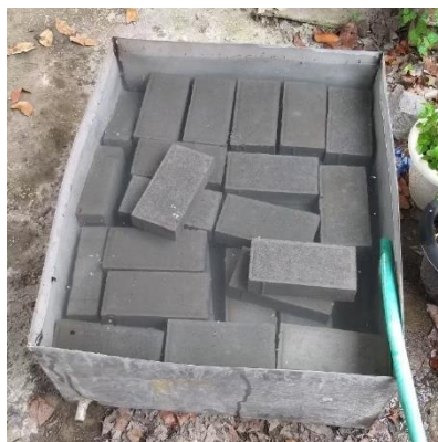
Lampiran L-4. 3 Perendaman Paving Block
