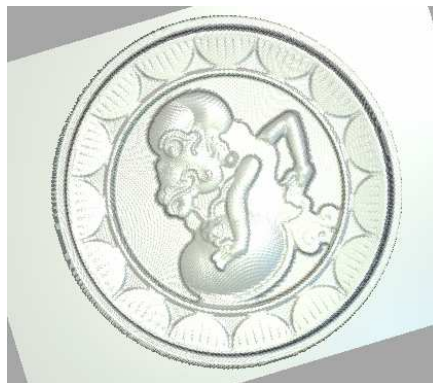
Gambar 4.7 Simulasi Proses Roughing
