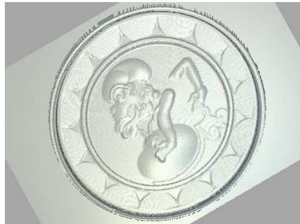
Gambar 4.11 Simulasi Proses Roughing
