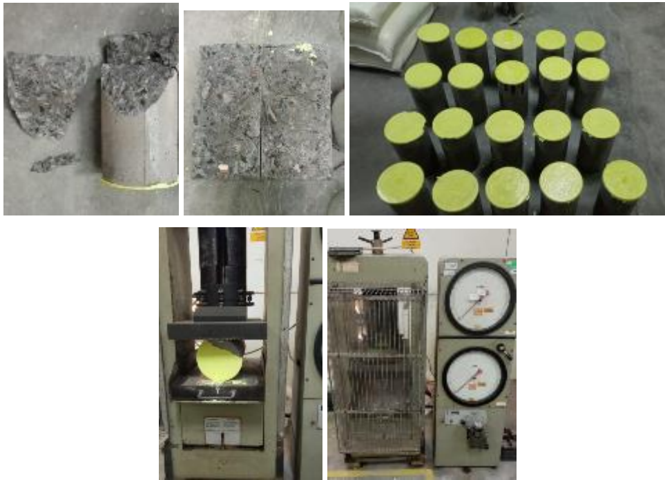
Figure 5.11 Tensile Test Process
