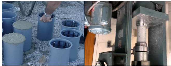
Figure 4.3 Compressive test (samples production and test)
