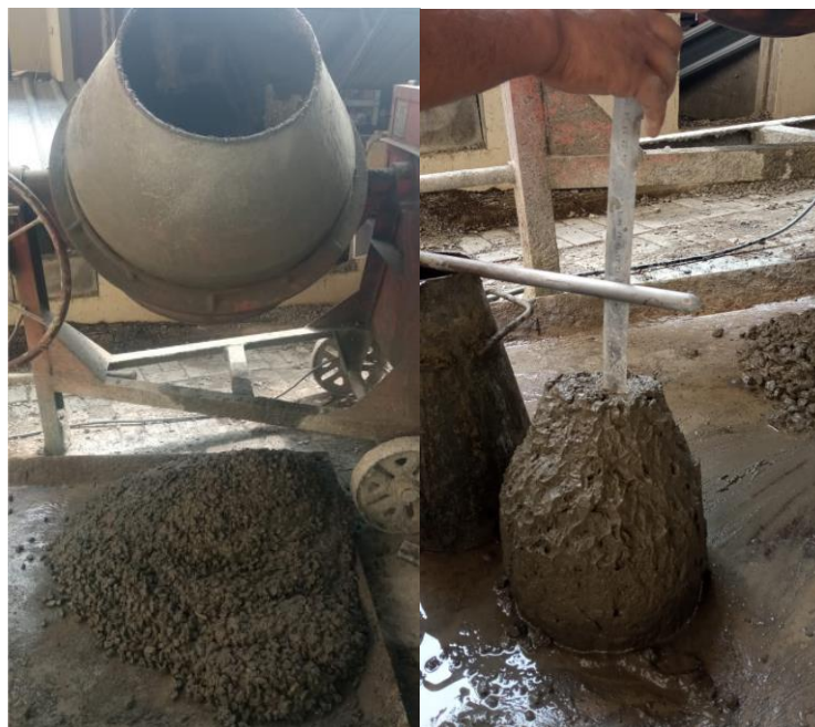
Figure 5.4 Mixing The Raw Materials and Slump Test
