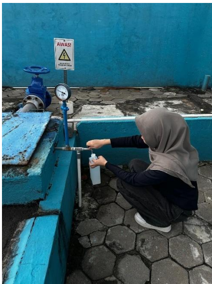
Pengambilan Sample Uji Coliform
