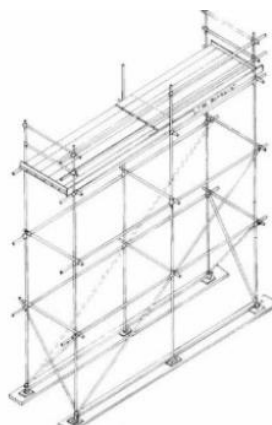
Gambar 3.13 Tube and Coupler Scaffolding
