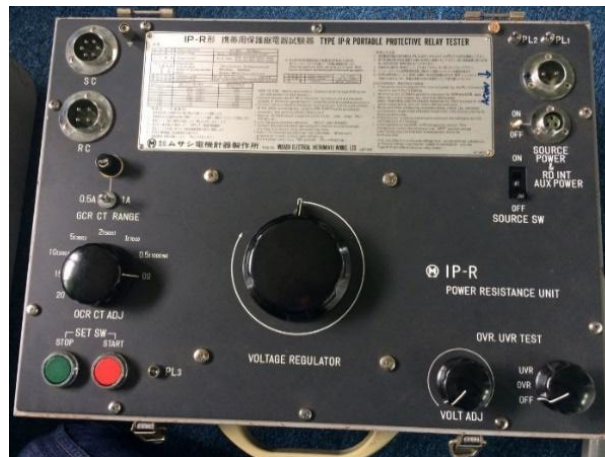
Gambar 3.2 Portable relay tester voltage regulator.
