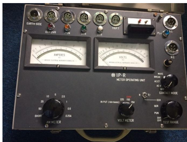
Gambar 3.3 Portable relay tester meter operating unit.
