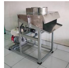
Porang chopper machine Dimensions: Height 130 cm Length and width 60 cm Capacity: 500 kg – 1000 kg/hour Source: shopee
