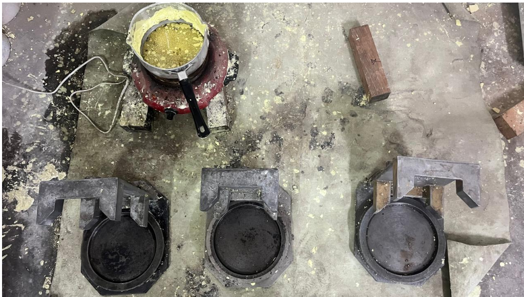
Gambar L-10.9 Proses Capping Benda Uji Silinder
