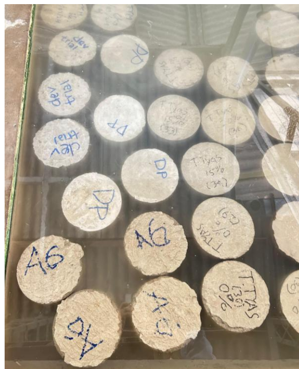
Gambar L-10.8 Proses Curing Beton kedalam bak perendaman
