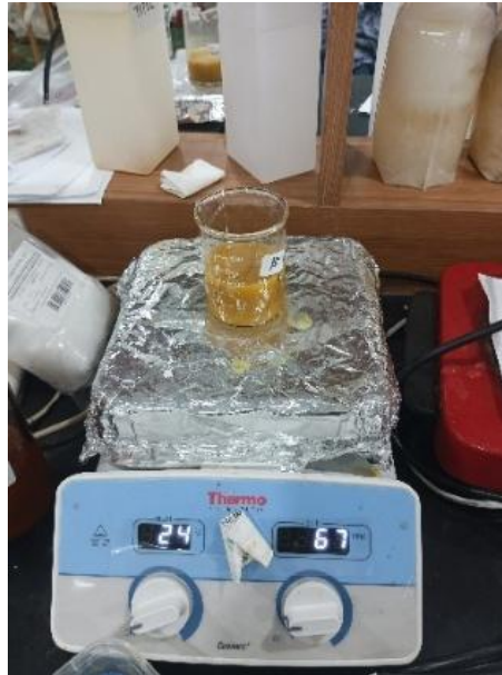
Gambar 3. 57 Proses Finishing Antibakteri Dip Coating
