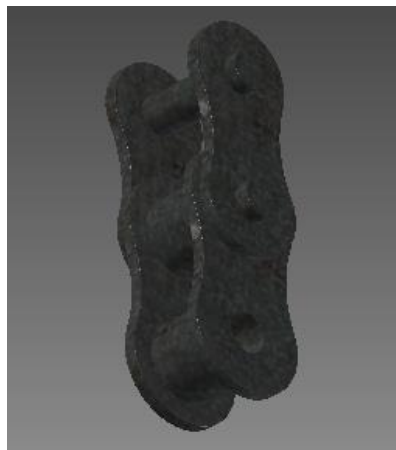
Figure 4.7 Roller chain RS-80 assembly pin & link
