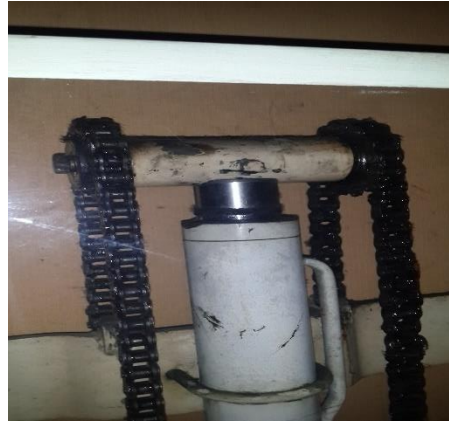
Figure 3.4 Example Assembly sprocket and chain
