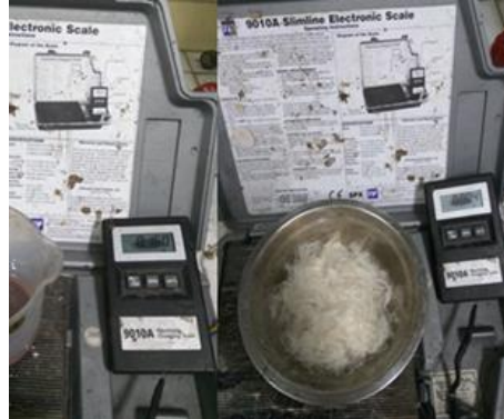
Gambar 3.41 Penimbangan Fiberglass, Bulu Ayam, dan Resin
