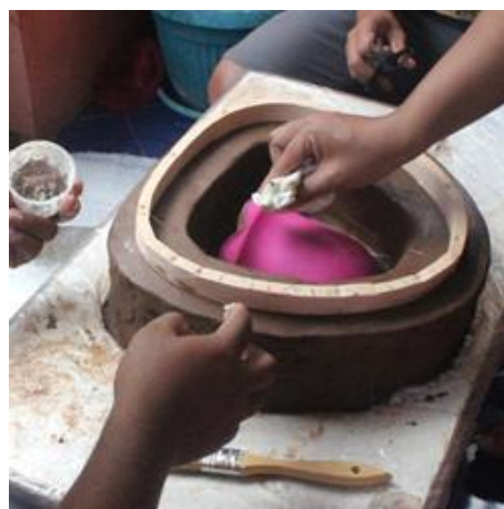
Gambar 3.24 Pengolesan Release Agent
