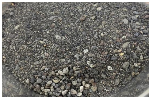
Gambar 4.2 Agregat Halus Pasir Pantai Pandansimo
