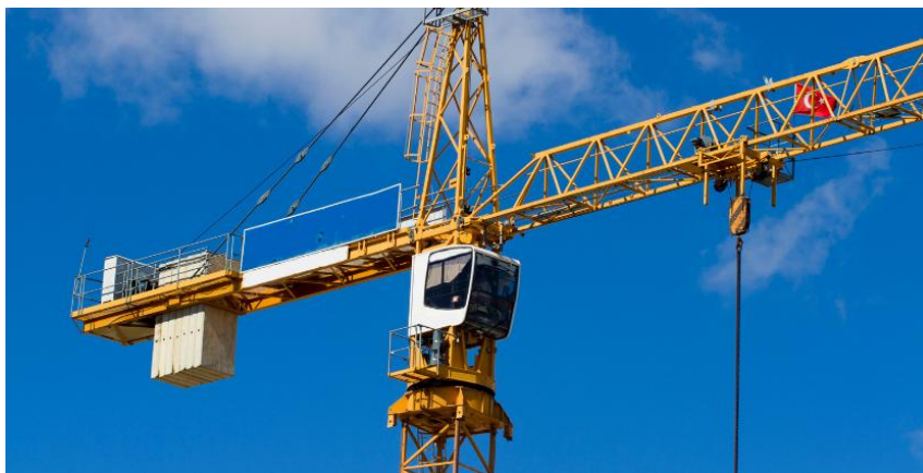
Figure 3. 2 Tower Crane (Sources: Google)
