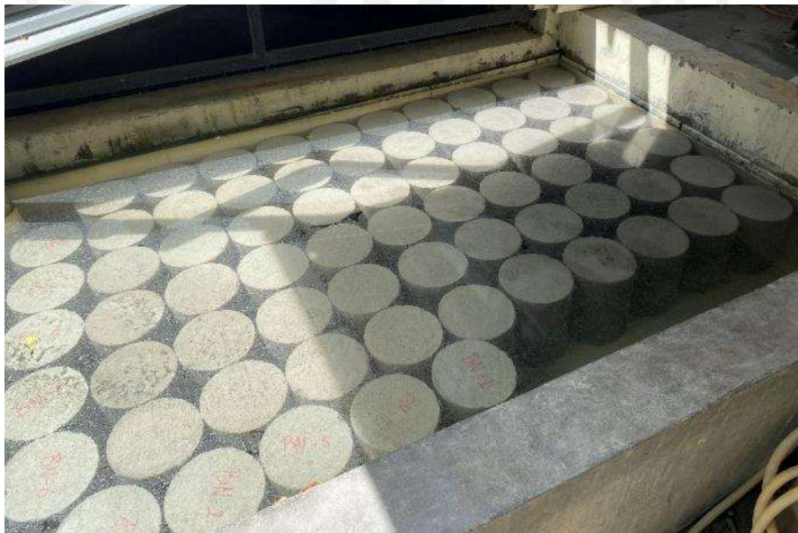
Gambar L-8.4 Proses Curing Silinder Beton
