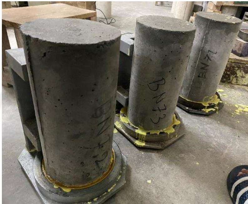
Gambar L-8.7 Proses Kaping Beton Silinder
