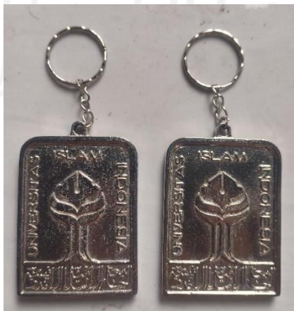
Gambar 4-19 Hasil Finishing Krom Nikel (Logo UIN)
