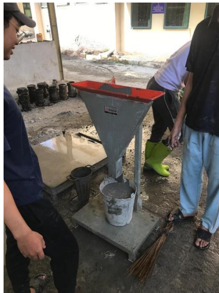
Gambar Lampiran 8.8 Proses Pengujian V-funnel
