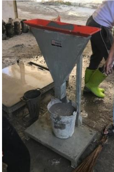
Gambar 5.10 Pengujian V-Funnel SCC
