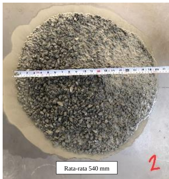
Gambar 5.6 Pengujian Slump-flow Trial 2
