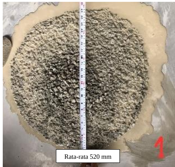
Gambar 5.5 Pengujian Slump-flow Trial 1
