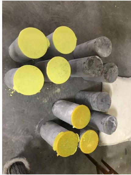
Gambar Lampiran 8.11 Proses Caping Beton
