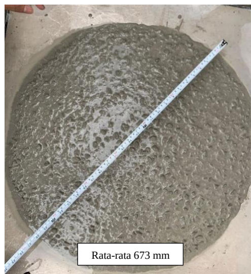
Gambar 5.9 Pengujian Slump-flow SCC
