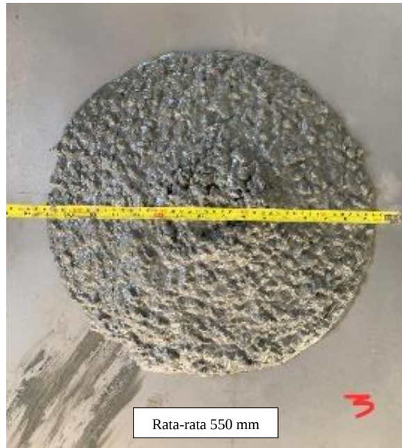
Gambar 5.7 Pengujian Slump-flow Trial 3
