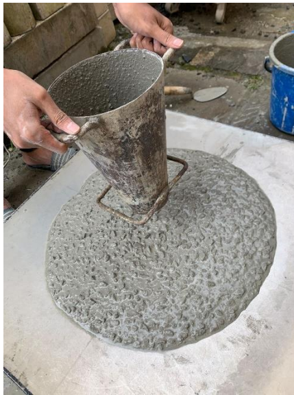
Gambar Lampiran 8.6 Proses Pengujian Slump-flow
