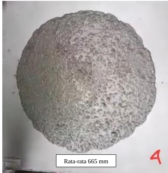
Gambar 5.8 Pengujian Slump-flow Trial 4
