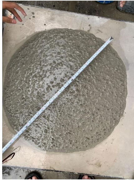
Gambar Lampiran 8.7 Hasil Pengujian Slump-flow
