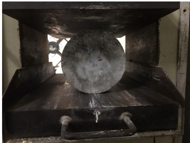
Gambar Lampiran 8.14 Proses Pengujian Kuat Tarik Beton
