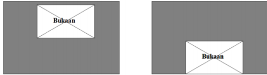
Fig. 3 Irregularity of Diaphragm Discontinuity
