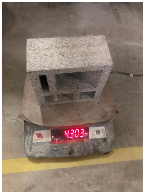
Gambar 4. 14 Roster Beton Motif Lubang 4 Sesudah Oven
