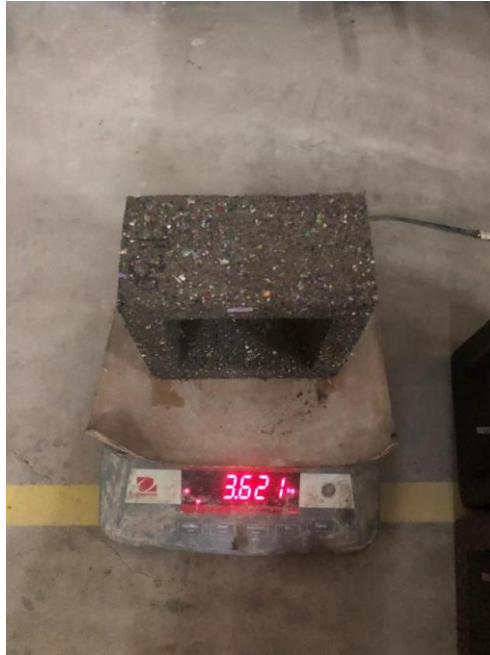
Gambar 4.10 Roster Beton Motif Lubang 1 Sesudah Perendaman
