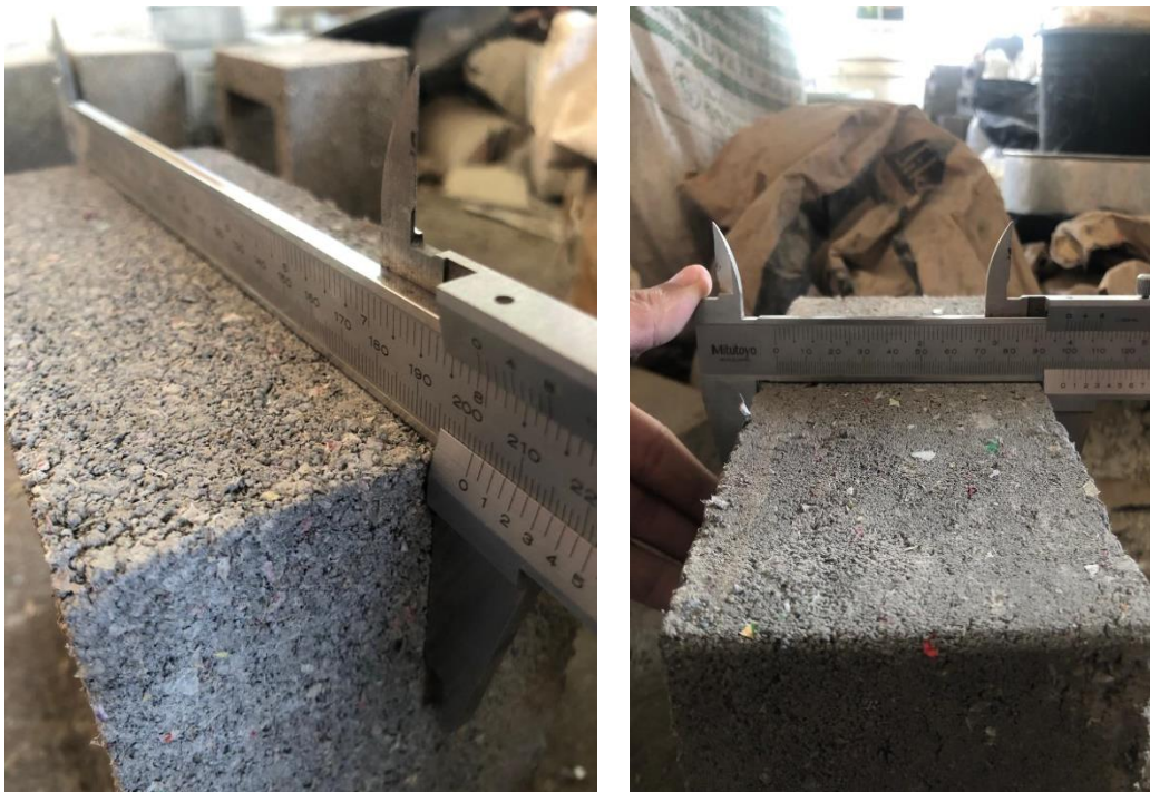
Gambar 4.3 Pengukuran Roster Beton
