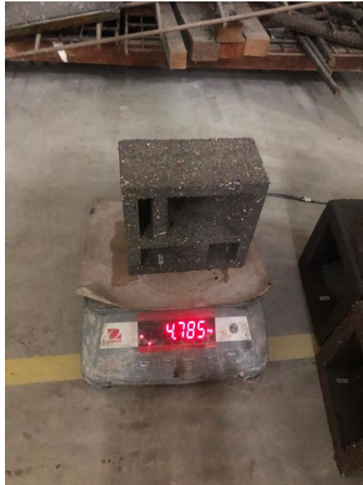
Gambar 4. 13 Roster Beton Motif Lubang 4 Sesudah Perendaman
