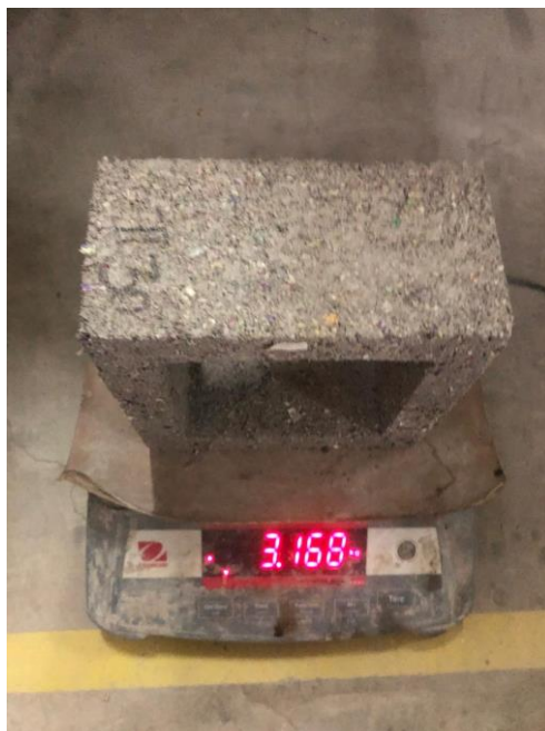
Gambar 4.11 Roster Beton Sesudah Di Oven Motif Lubang 1
