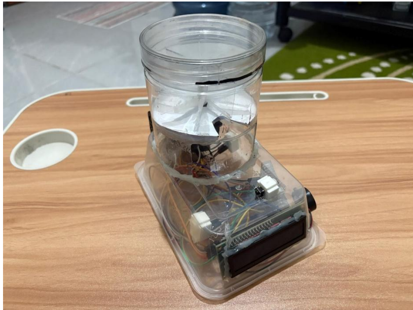
Gambar 4.1 Prototipe Fungsional Dispenser Obat.
