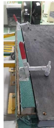
Gambar 5. 4 Stoper Meja Vertical Sander Key bed After
