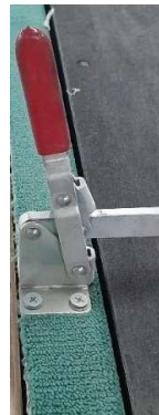
Gambar 5. 3 Stoper Meja Vertical Sander Key bed Before
