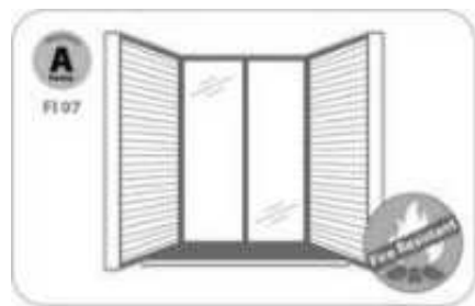
Figure 58. Fire resistant window shutters
