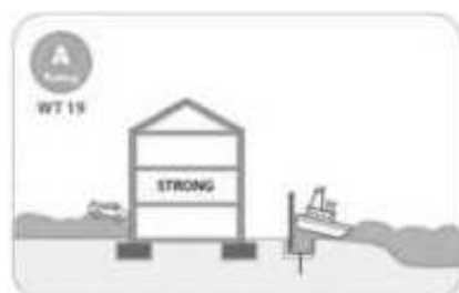
Figure 47. Building structure to withstand water-borne debris damage
