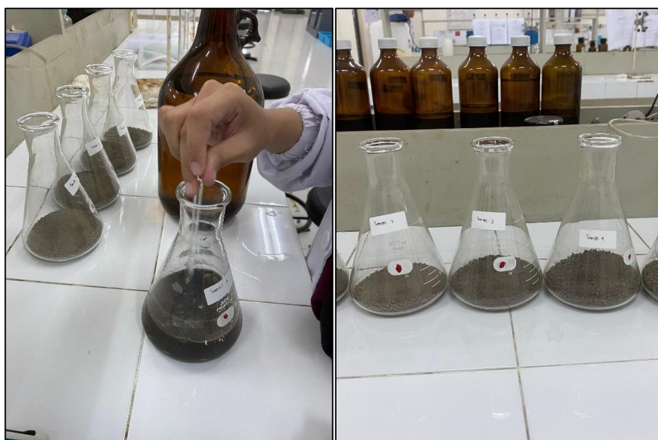
Gambar 3.6 Proses Density Separation
