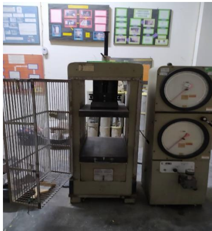
Gambar L-3.13 Compressing Testing Machine (CTM)
