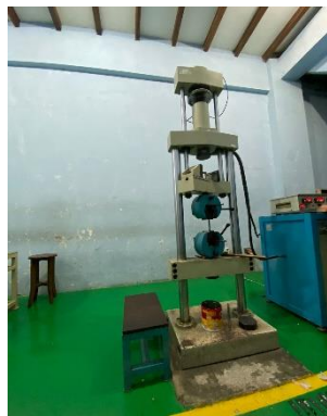
Gambar 3- 9 Mesin UTM ( Universal Testing Machine ).
