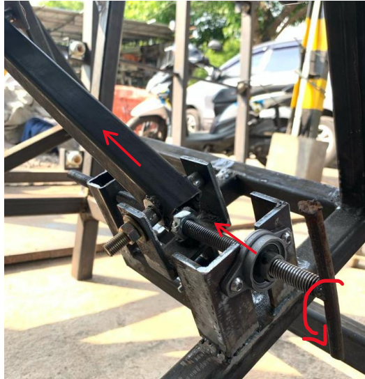
Gambar 4 - 41 Trial and Error Mekanisme Lift
