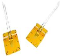
Gambar 4.28 Strain Gauge Uji Tekan Rangka Atap
