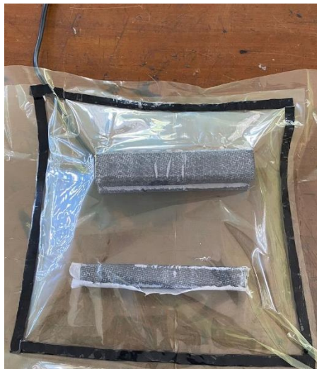
Gambar 3. 25 Rangkaian Vacuum Bagging
