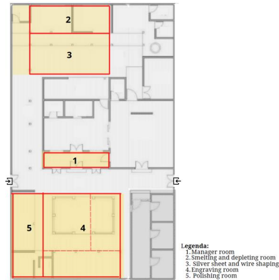
Figure 4.3 Division of Spaces in Workshop Zone After Renovation (Image source: Author's direct observation)
