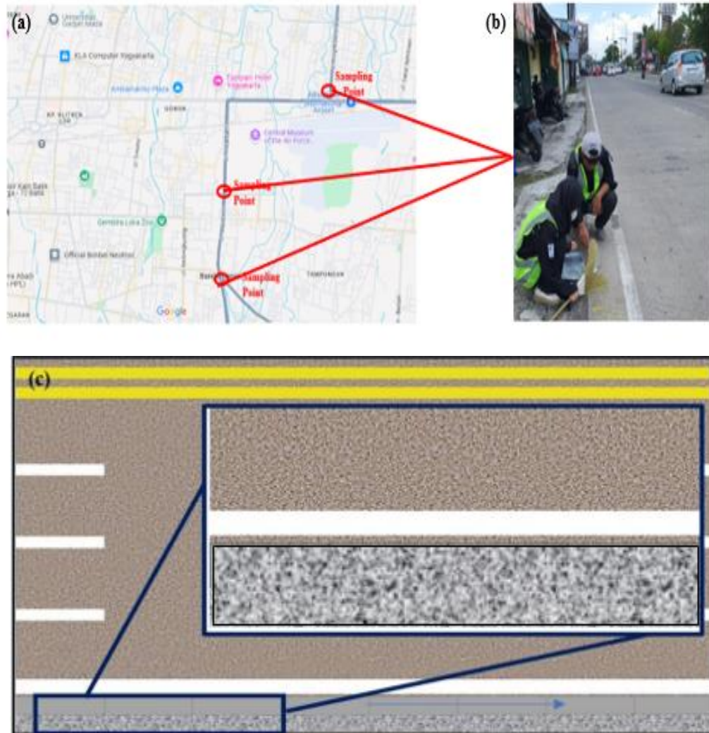
Gambar 3.4 Metode Pengambilan Sampel Debu Jalanan; (a) Titik Sampling, (b) Pengambilan Sampel, (c) Lokasi Pengambilan Sampel Debu Jalanan
