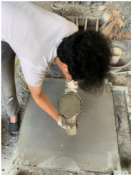
Gambar Lampiran 5.4 Pengujian Slump-flow
