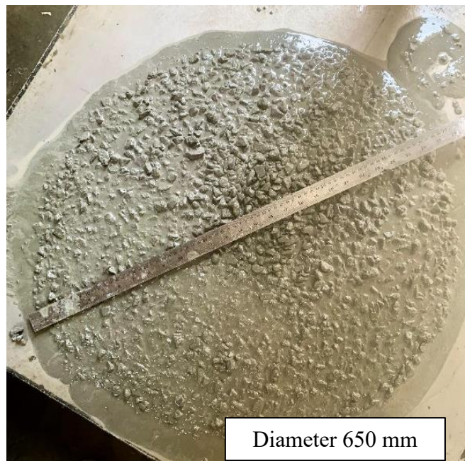
Gambar 5. 6 Pengujian Slump Trial 4
